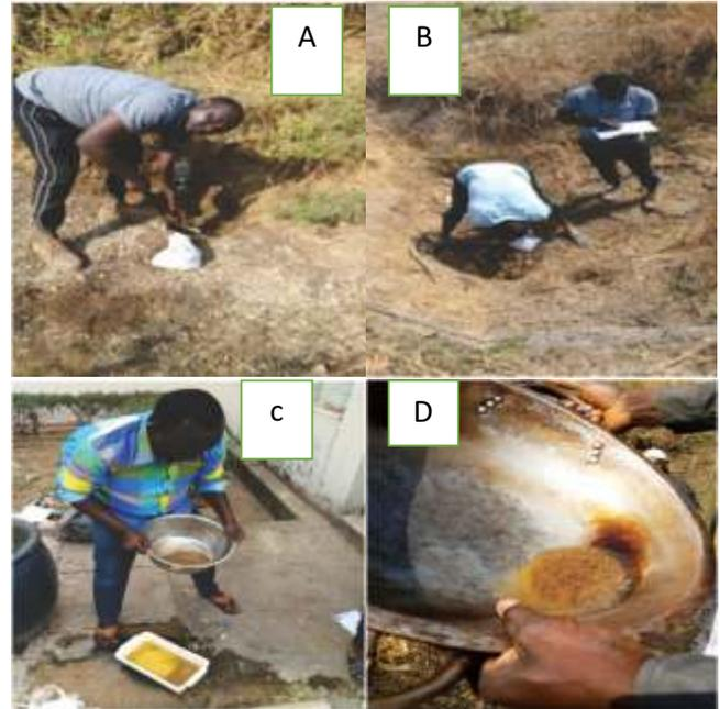
Plate 1: (a) collection of sample on the field (b) recording of field observation (c) panning of stream sediment sample to separate coarse sediment from the suitable one (d) pan concentrate of gold grains
