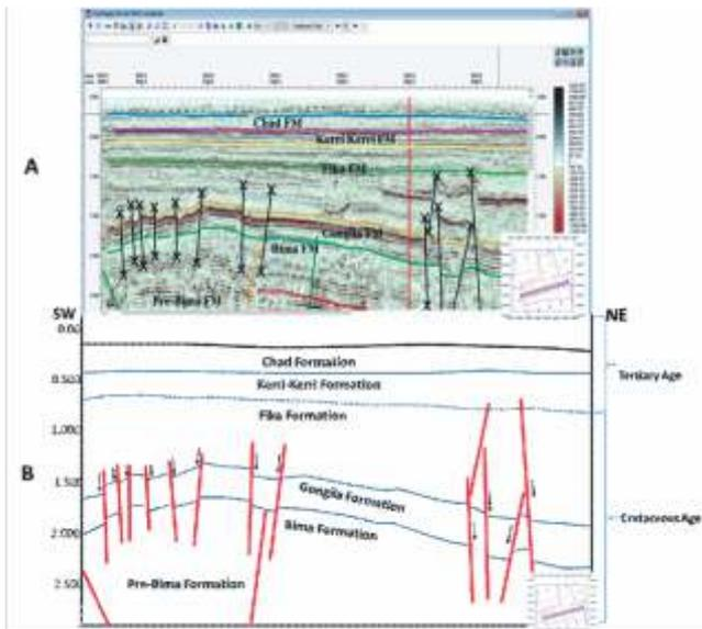
Figure 7: NE-SW seismic section (A) and its interpreted geologic equivalence (B)
