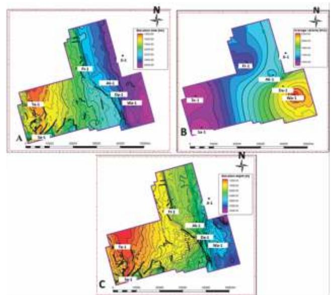
Figure 9: (A) Time structure map of top of Gongila Fm. (B) Average velocity map (C) Depth structure map using Average Velocity function.
