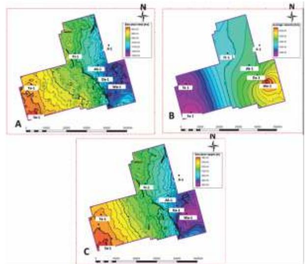
Figure 8: (A) Time structure map of top of Kerri-Kerri Fm. (B) Average velocity map (C) Depth structure map.
