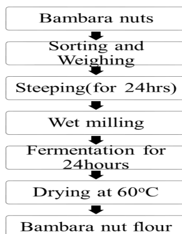
Figure 2: Flowchart for the Production of Bambara nut Flour
