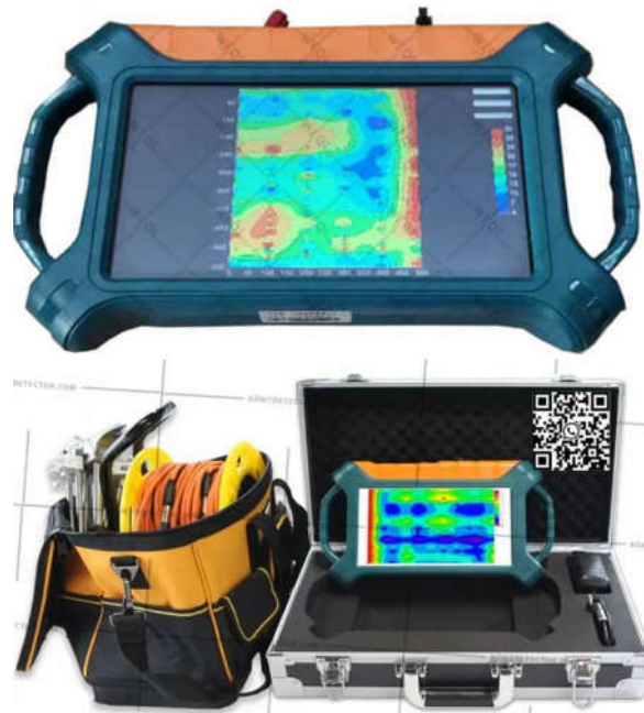
Fig. 3: SAS 300 ADMT Survey equipment and its accessories
