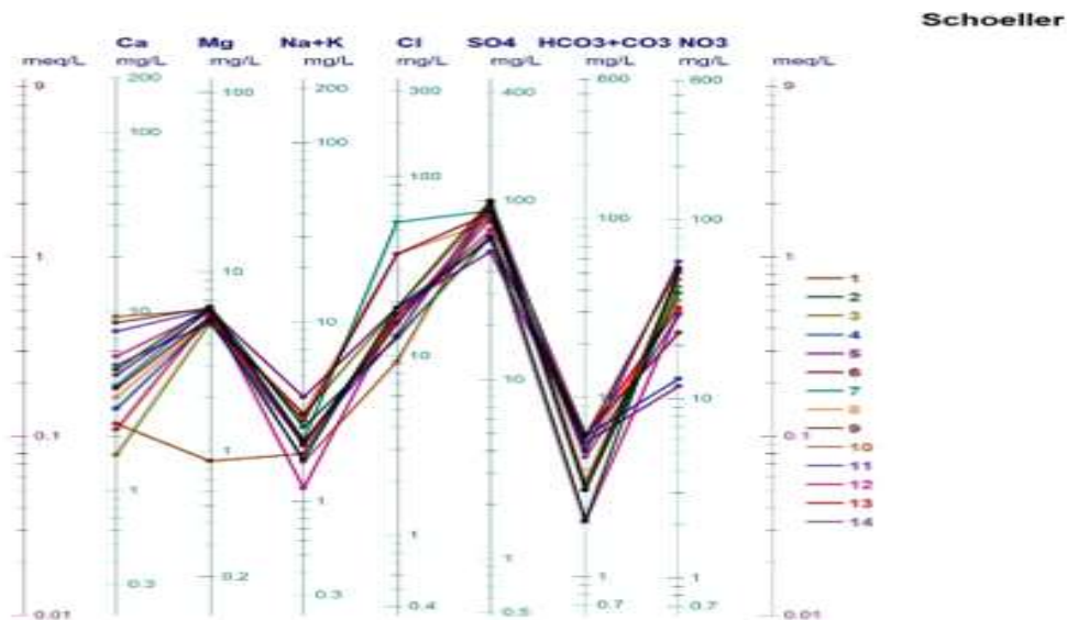
Figure 6: Schoeller diagram showing groundwater evolution
